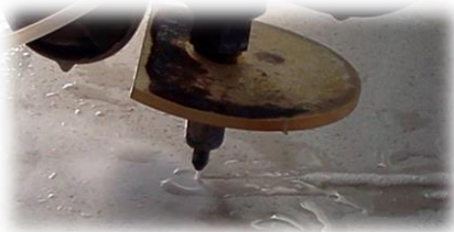
Cut-out by water jet
