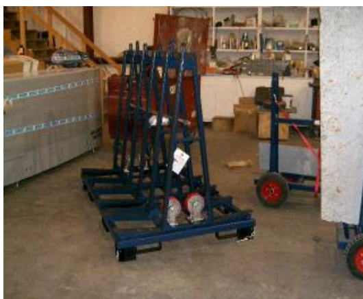
Rack for easy access & also mountsto a flatbed truck
