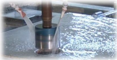
Wet drilling with core bit
