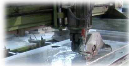
Cutting with bridge saw
